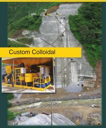
This is an example showing the custom capabilities available from ChemGrout. The fully automated CG690/ES was designed for the Cachi Hydroelectric Dam Project in Costa Rica. Drawing on over 50 years of experience, this unique design provides high shear colloidal mixing, high material outputs, and extremely accurate mix ratios.
